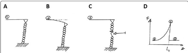
**Figure 3 Force spectroscopy of a single polymer by Atomic Force Microscopy**. (A) The polymer ends are grafted to a surface and to the cantilever; (B) the surface is lowered thereby causing the bending of the cantilever; (C) A domain (shown by the arrow) is opening and the cantilever returns to its original position; (D) The corresponding force-extension curve is shown.
