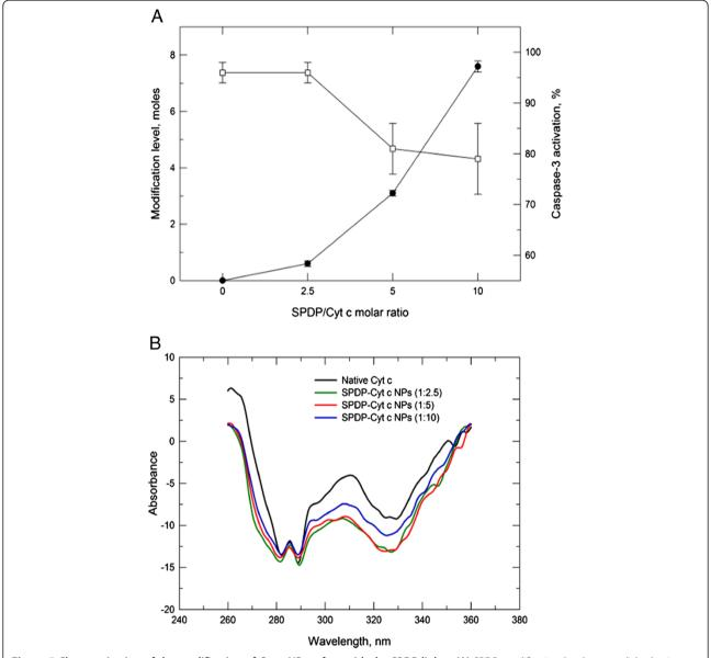
**Figure 5** Characterization of the modification of Cyt c NP surface with the SPDP linker. (A) SPDP modification level accomplished using increasing reagent concentrations during synthesis (closed symbols) and effect of the modification on *in vitro* caspase-3 activation in a cell-free system (open symbols). (B) Near-UV CD spectra of dissolved Cyt c NPs after modification with SPDP.
