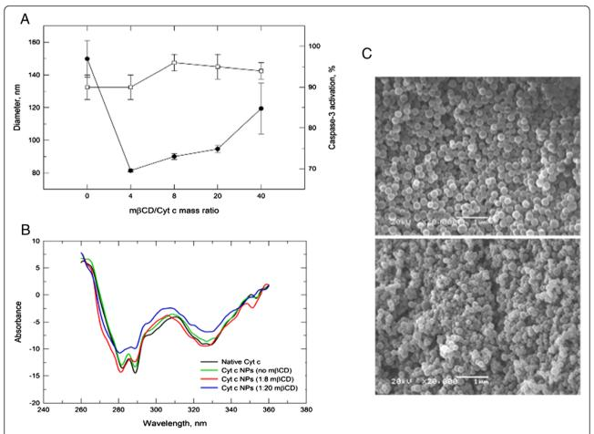
Figure 3 The effect of methyl- $\beta$ -cyclodextrin (m $\beta$ CD) during the protein precipitation. (A) Effect of m $\beta$ CD on the particle diameter ( $-\bullet-$ ) and caspase-3 activation ( $-\Box-$ ) after Cyt c nanoprecipitation. (B) Near-UV CD spectrum of Cyt c nanoprecipitated in absence or presence of m $\beta$ CD. (C) SEM image of Cyt c NPs made without m $\beta$ CD (upper picture), and at a 1:8 Cyt c-to-m $\beta$ CD mass ratio (lower image).
