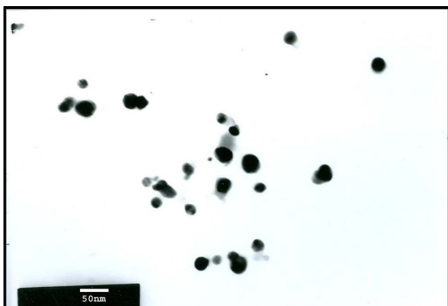
Figure 1 TEM images obtained from purified fractions collected after sucrose density gradient of Ag-NPs synthesized using B. licheniformis . Purified nanoparticles from B. licheniformis were examined by electron microscopy. Several fields were photographed and were used to determine the diameter of nanoparticles. The range of observed diameters is 50 nm.
