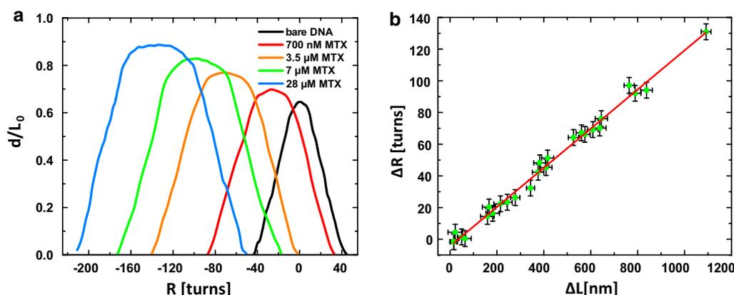
**Fig. 3** **a** Results of single DNA molecule overwinding experiments with stepwise increased MTX concentration at a preset force of 0.2 pN; **b** plot of the change of the rotation number  $\Delta R$  with corresponding elongation of the DNA contour length  $\Delta L$ . The slope (linear approximation, solid line) allows estimating the unwinding angle per intercalated MTX molecule
