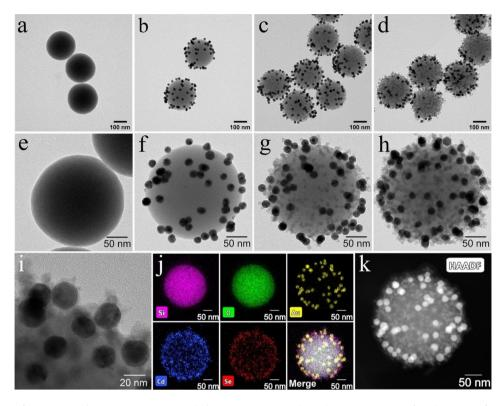
Fig. 1 TEM images of (a) SiO<sub>2</sub> core, (b) Si-Au, (c) Si-Au/QD, and (d) Si-Au/DQD NPs. High-resolution TEM images of single (e) SiO<sub>2</sub>, (f) Si-Au, (g) Si-Au/QD, and (h) Si-Au/DQD NP. (i) TEM image of Si-Au/DQD with local enlargement. (j) EDS elemental mapping images of a single Si-Au/DQD NP. (k) HADDF image of a single Si-Au/DQD NP.
