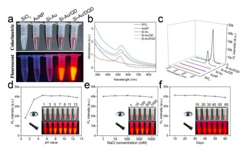
Fig. 2 (a) Photographs of SiO<sub>2</sub>, AuNP, Si-Au, Si-Au/QD, and Si-Au/DQD under visible and UV light. (b) UV-vis spectra of these NPs. (c) Fluorescence spectra of these NPs. Stability of Si-Au/DQD under pH (d), salt (e), and time (f) conditions
