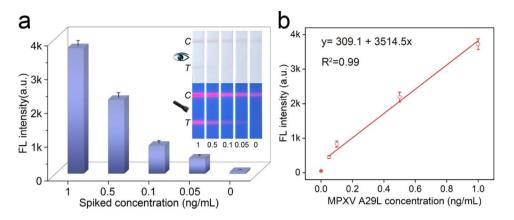
Fig. 6 (a) Colorimetric/fluorescent images of the strips and the corresponding T-line signal intensities for MPXV detection (1-0.05 ng/mL). (b) The linear relationship of the fluorescence signals with MPXV concentrations
