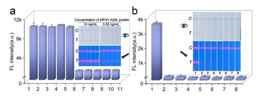
Fig. 5 (a) Reproducibility of Si-Au/DQD-based LFIA. (b) Specificity of Si-Au/DQD-based LFIA. The numbers 1–8 at the bottom of the strip represent the detection targets of MPXV (1ng/mL), VCAV (100 ng/mL), CPXV (100 ng/mL), VZV (100 ng/mL), SARS-CoV-2 (10<sup>6</sup> pfu/mL), FluA (10<sup>6</sup> pfu/mL), FluB (10<sup>6</sup> pfu/mL), and HAdV (10<sup>6</sup> pfu/mL)
