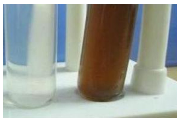
Figure 1 1 mM silver nitrate solution without callus extract and silver nanoparticles with reddish brown colour. 1 mM silver nitrate solution without callus can be seen in A and silver nanoparticles with reddish brown colour can be seen in B.
