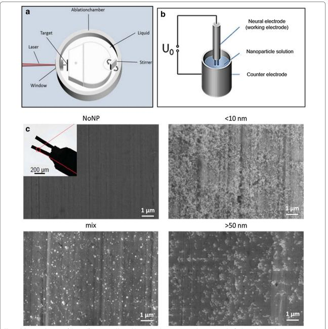
Fig. 2 Schematic drawings of the a self-constructed laser ablation chamber to generate the nanoparticles, b electrophoretic deposition set-up to coat the electrode surface, and c exemplary SEM-images of the uncoated and coated contact surfaces (nanoparticles smaller than 10, 50 nm and mixture of both)
