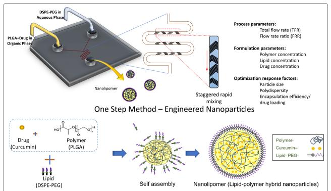
**Fig. 1** Schematic diagram of synthesis process. Staggered herringbone based microfluidic chip for synthesizing the nanolipomer nanoparticles. The PLGA + drug core is formed by nano-precipitation in the microfluidic chip and introduced from one inlet while the DSPE-PEG lipid coating is injected from the opposite port. The final nanolipomer is collected in the third port after rapid mixing has occurred
