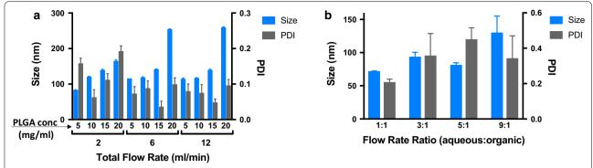
**Fig. 2** Instrument parameters optimization. **a** Effect of total flow rate (TFR) on the size and polydispersity (PDI) of the nanolipomers at polymer concentration of 5, 10, 15, and 20 mg/ml (DSPE-PEG concentration = 40%, aqueous:solvent FRR = 1:1). **b** Effect of aqueous:solvent flow rate ratio (FRR) on the size and polydispersity (PDI) of nanolipomers at polymer concentration of 10 mg/ml (DSPE-PEG concentration = 40%, TFR = 12 ml/min). (n = 3: mean ± SD)
