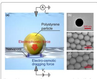
**Fig. 1** a Schematic image of nanopore trapping method and **b-d** scanning microscopic images of pore and particles. **b** A 600 nm-sized nanopore was employed for capturing carboxylated-polystyrene particles sized **c** 780 nm and **d** 900 nm
