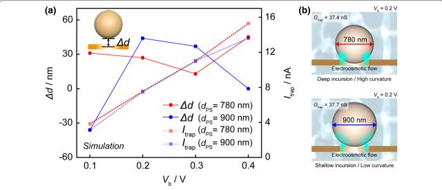
Fig. 4 a Particle positions and ionic currents in trapping derived from multiphysics simulations. **b** The commensuration between contribution of particle curvatures and positions at  $V_h = 0.2$  and 0.3 V
