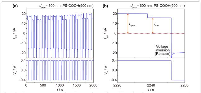
**Fig. 2** a Typical consecutive current traces of electrophoretic particle trap and **b** magnified view of a single trace showing open pore current  $I_{\text{open}}$  and suppressed  $I_{\text{trap}}$ . Trapping/detrapping processes are controlled by inversion of  $V_{\text{b}}$
