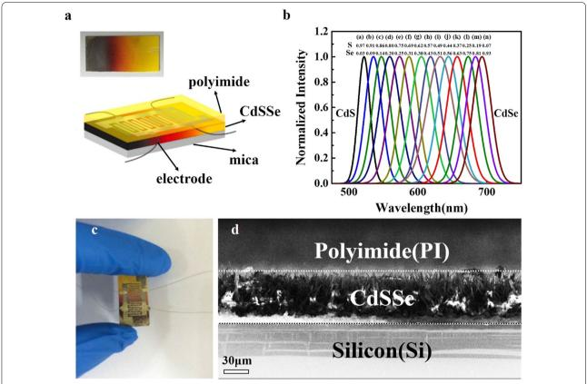
**Fig. 1** a Real-color photograph of tunable-composition ternary alloy  $CdS_{1-x}Se_x$  chip and the diagram of the sweat sensor. **b** PL spectra measured at different composition along the length direction of the CdSSe nanowire chip by a laser at 405 nm. **c** Real image of the as-prepared sweat sensor. **d** Cross-sectional SEM image of silicon (Si) substrate based Pl-coated CdSSe nanowire chip. Scale bar: 30  $\mu$ m
