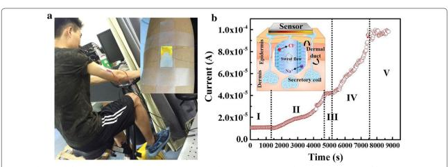
Fig. 5 a Photograph for real-time on-body sweat monitoring during indoor cycling. The inset: real-time monitoring scene of the sensor attaching to the arm. b The data of real-time skin sweat measurement. The inset: schematic diagram of sweating monitoring for sensor attaching to the skin
