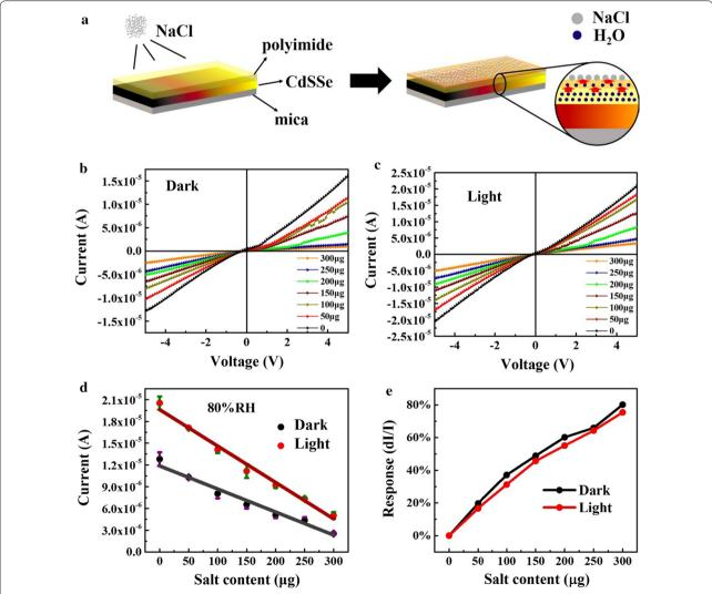
Fig. 3 a Salt-sensing process and mechanism of a CdSSe-based sensor. I–V characteristic curves of salt sensing in the dark (b) and light (c) under different salt content levels at high humidity of 80% RH. d The current variation of the sensor with the salt content at a bias of 5 V. e The salt content dependent responsivity of the CdSSe-based sensor
