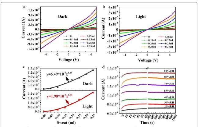
**Fig. 4** I-V curves of the sensor under different amounts of human sweat in the dark (**a**) and bright (**b**) fields, respectively. **c** Conductive currents under dark and light condition are shown to directly correlate with sweat volume, underscoring the possibility of quantitative analysis of sweat monitoring. The corresponding regression curve was given to predict the volume of sweat by the current of the sensor. **d** Long-term stability of the CdSSe nanowire-chip sensor
