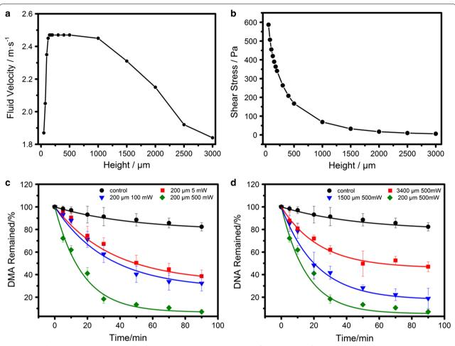
**Fig. 3** Tunable DNA release. Variation trends of maximum vortex speed (**a**) and interface shear stress (**b**) when changing the height were theoretically analyzed using FEM simulation. Experimental release effectiveness under different power (**a**) and height (**b**) were recorded using percentage of remained DNA as a function of resonator treating time, observed at 0, 5, 10, 20, 30, 50, 70 and 90 min
