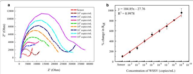
**Fig. 3** WSSV detection using the disposable electrode. **a** Nyquist plots for different concentrations of WSSV in the range of  $10^2-10^9$  DNA copies/ml. **b** Calibration curve of the corresponding impedance. Each detection was performed three times and data are given as average  $\pm$  SD (n = 3)
