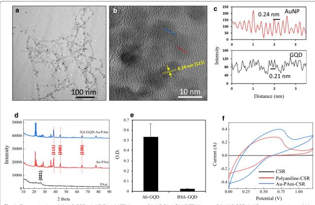
**Fig. 1** Characterization of Ab-N,S-GQD@AuNP-PAni. (a) TEM image of AuNP-PAni, (b) HR-TEM image of the N,S-GQD-AuNP nanocomposite, and (c) fringe analysis using ImageJ. (d) Powder XRD analysis of silicon, PAni/CSR, AuNP-PAni/CSR, and N,S-GQD-AuNP-PAni/CSR. (e) ELISA of Ab-N,S-GQDs. (f) Cyclic voltammetry diagrams of CSR, polyaniline-CSR and AuNP-PAni/CSR
